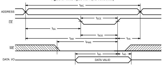
Figure 7. Write Cycle No. 2 (WE Controlled, OE HIGH during Write) [14, 15]
