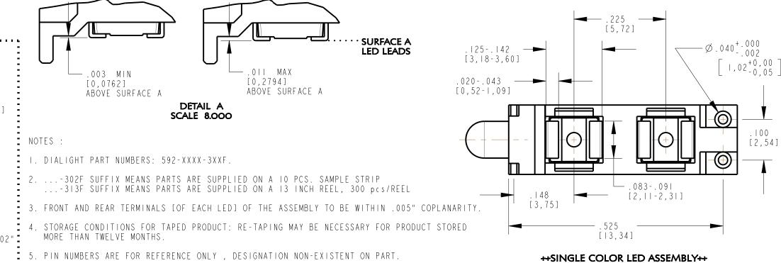
6. MOISTURE SENSITIVITY LEVEL LABEL WILL BE PLACED ON BAG. CHECK CHART FOR PROPER LEVEL. 7. THIS ASSEMBLY CONTAINS ELECTROSTATIC DISCHARGE SENSITIVE DEVICES (ESDS). MAINTAIN ALL PRECAUTIONARY MEASURES DURING ASSEMBLY, HANDLING, AND STORAGE IN ACCORDANCE WITH IPC-A-610.
