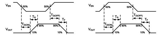
Figure 1. Voltage Waveforms: AP2145 (left), AP2155 (right)
