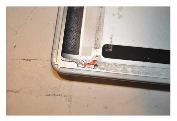
Next, place the screen into the back panel, and observe where the ribbon cable will need to exit the case. You will need to make a cut with your Dremel to pass this cable through the case, and out to the Qualia board.
