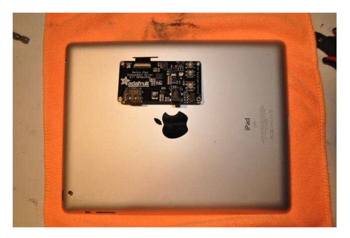
Now, use your fine tipped marker to mark where the mounting holes line up. Another method is to place the board on an 8x11 sheet of paper, and create a drilling stencil. Then, hold the back panel up to the head of your lamp, and mark where you need to drill the holes for the lamp mount. The ideal place for the lamp is not dead center, but slightly offset towards the side with the rear facing camera.
