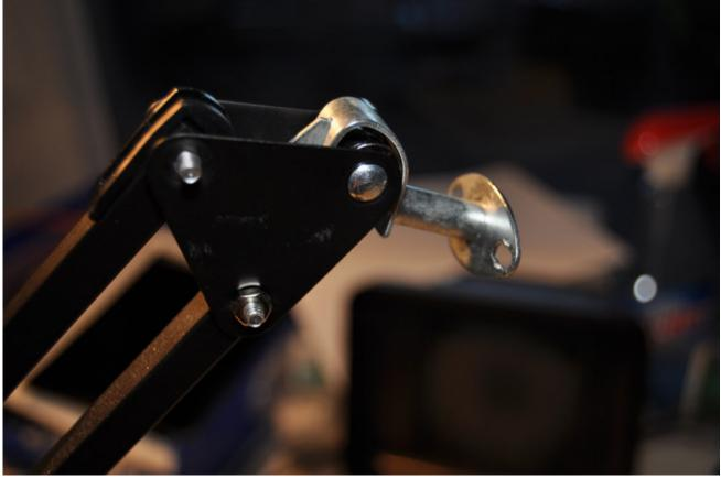
Awesome! I'd save the head of the lamp for another cool project. We won't need it here! Last bit for the lamp for now. The oval bracket that was holding the head before is slightly curved (to be flush with the lamp head), so use your needlenose pliers and straighten it out.
