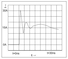
Figure 18. ESD Test Waveform for IEC61000-4-2
