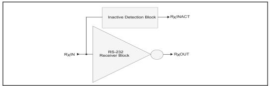
Figure 14. Stage I of AUTO ON-LINE® Circuitry
