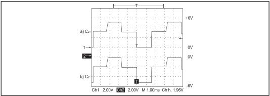
Figure 10. Charge Pump Waveforms
