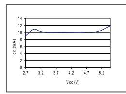
Figure 2. Supply Current VS. Supply Voltage
