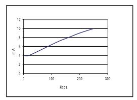
Figure 4. Supply Current VS.Data Rate
