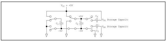
Figure 11. Charge Pump - Phase 3
