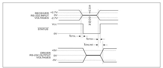
Figure 13. AUTO ON-LINE® Timing Waveforms
