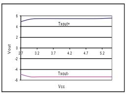
Figure 3. Transmitter Output Voltage VS. Supply Voltage
