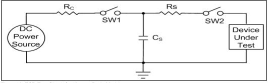
Figure 16. ESD Test Circuit for Human Body Model
