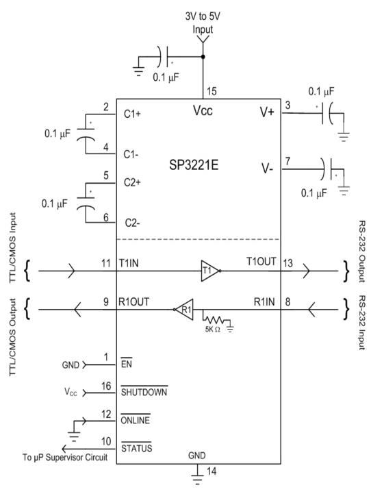
Figure 1. SP3221E Typical Operating Circuit
