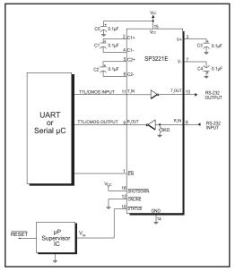
Figure 5. Interface Circuitry Controlled by Microprocessor Supervisory Circuit
