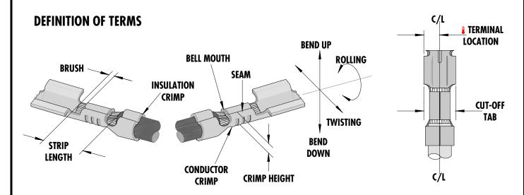
Iterminal is to be centrally located between the two (2) cut-off tab edges by one half of the total cut-off tab tolerance. This illustration is a generic terminal representation and not an exact image of any terminal listed in the scope.
