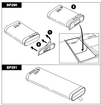
The BP291 does not need any modification before you install the battery pack into the test tool.
